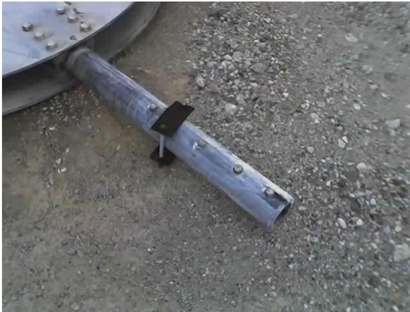
Photo of fan hub and steel spar (connecting shaft for Al Blade)
